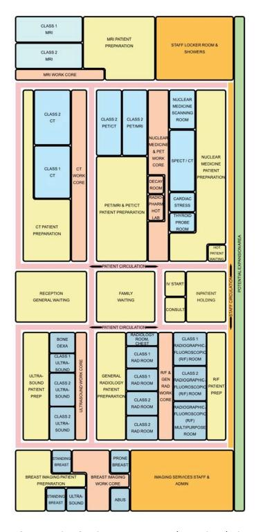
Figure 3.1: Imaging Services Departmental Functional Diagram.
