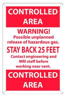
Figure 2.7.3.3-3: Example of warning signage text to be placed near quench pipe discharge or around the exclusion zone perimeter.
